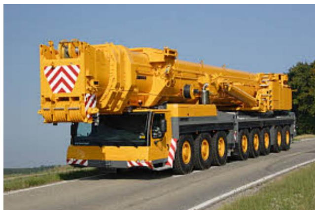
Plate 3.5: Crane for wind turbine erection 2
